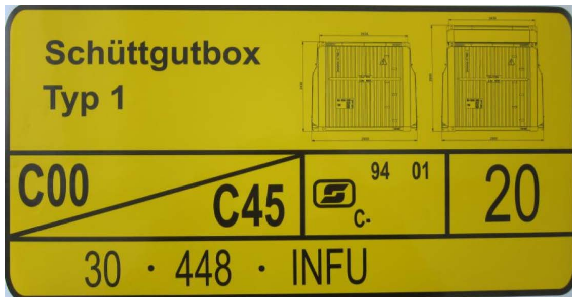
Example: yellow codification sign acc. UIC 596-6
