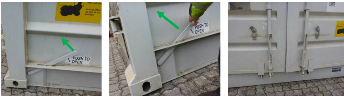
Figure 135: Type F, Opening back doors and flaps E.4.
