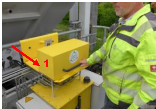
Figure 100: Type E, Adjustment of the baffle plate C.4.
