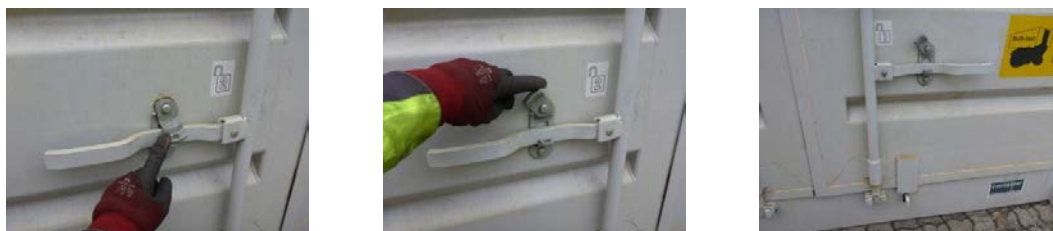
Figure 131: Type F, Opening the back flaps and doors E.2.
