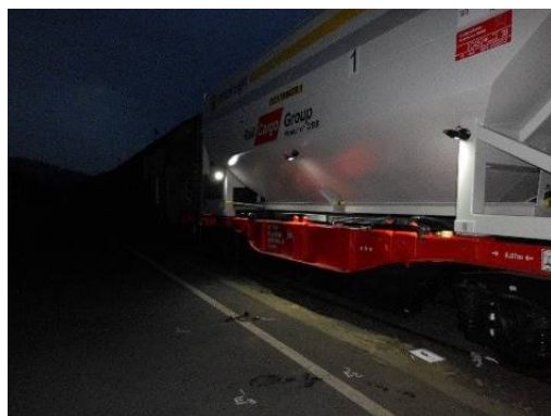
Figure 92: Type E, Attachment of hand lamps C.2.1.
