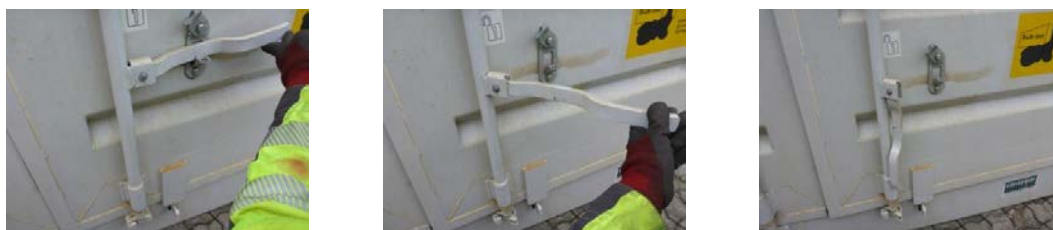
Figure 132: Type F, Opening the back flaps and doors E.3.
