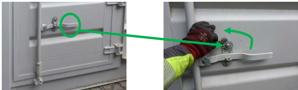
Figure 200: Type L, Open side door B.2.1.1.
