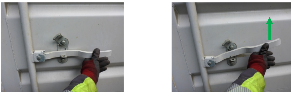
Figure 201: Type L, Open side door B.2.1.2.
